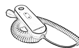
7. Handset with simple dry contacts
