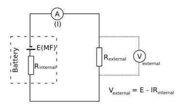
RInternal =  $20 \text{ m}\Omega$ E = 12 VDC4 x icon50: IDC = 120 ADCVinternal = 2,4 VDC (loss)
