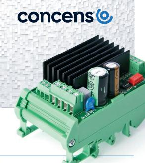
The C2-20 actuator controller provides advanced positioning and control of actuators through easy and flexible integration with the application. The controller is designed to work with Concens electrical in-line actuators in applications where positioning is required. C2-20 has adjustable start and stop ramps, which make smooth starts and stops possible. The C2-20 works in conjunction with actuators with hall only.
