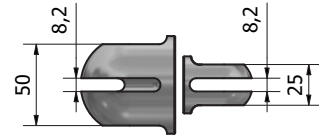
Alu/Stainless steel with clevis Max. static load 18100 N
