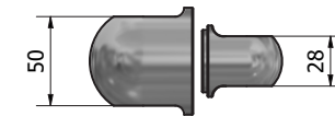
Alu with spherical bearings/ Stainless steel with stainless spherical bearings Max. static load 11000 N Max tilt 8°
